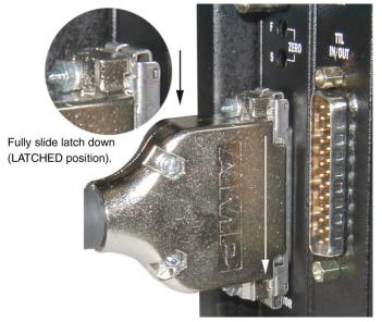
3. Verify that the connector is fully secured.
